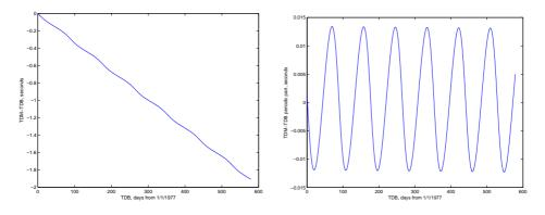
Figure 2: Left: TDM as function of TDB shows a drift due to the non-zero average of the 1-PN term. Right: the oscillatory term, with the period of Mercury's orbit, is almost an order of magnitude larger than TT-TDB.
