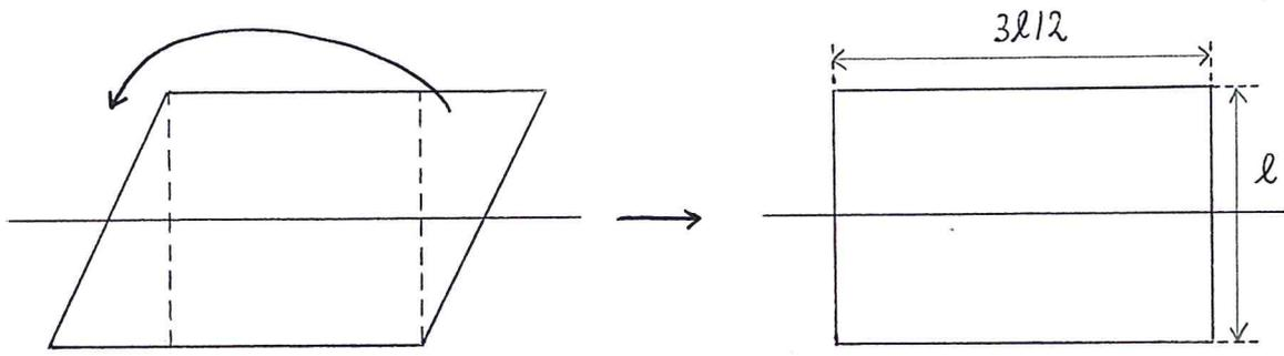
$$I_{Ox} = \sigma \int_{-l/2}^{l/2} \int_0^{3l/2} y^2 dx dy = \frac{3l\sigma}{2} \frac{1}{3} \left( \frac{l^3}{8} + \frac{l^3}{8} \right) = \frac{ml^2}{12}, \quad \sigma = \frac{2m}{3l^2}$$
